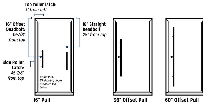
Offset pulls are designed to incorporate a deadbolt along the length of the pull, whereas a straight pull incorporates the deadbolt installation above the pull.
